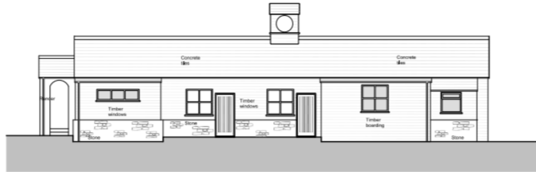
South West Elevation
